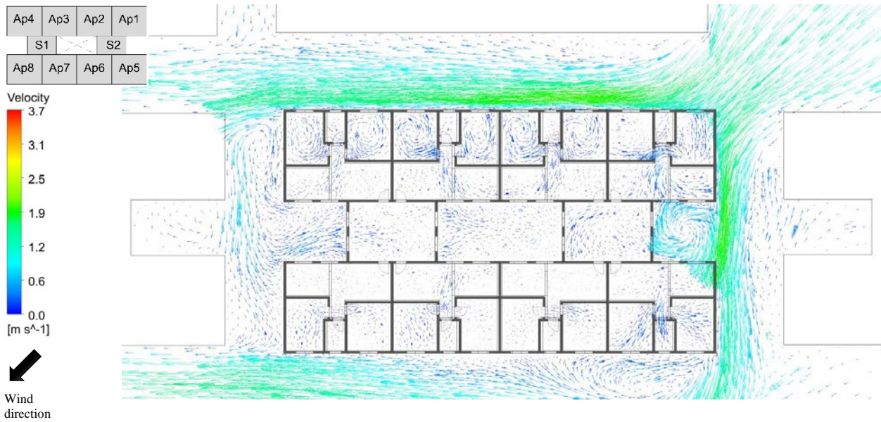
Figure 11. Airflow in the fourth floor apartments at wind attack angle of 45°, obstructed surrounding.
