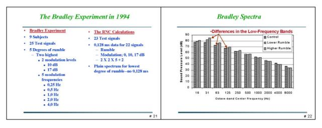
(SLIDE 22) The original two unmodulated rumble spectra used for the modulation experiment and the control signal spectra are shown here. The differences are in the low-frequency bands. Each of the 9 subjects compared separately each of the 24 test signals to the neutral, reference spectrum.
