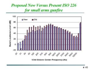
(SLIDE 45) The next slide shows a similar comparison for small arms gunfire. The previous 3 slides show that there is a big difference in the emphasis that the two sets of curves place on the low frequency energies. The current ISO 226 places a greater emphasis on the low frequency energies and, in terms of annoyance, it correlates very much better with subjective human response.
