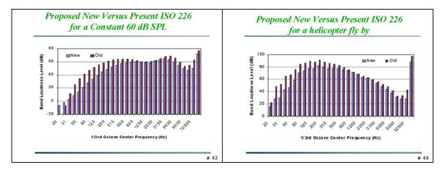
(SLIDE 44) This slide shows the (energy) time-integrated phon levels in each 1/3rd-octave band using both the current and the proposed ISO 226 curves for a helicopter fly by. The current procedure shows much higher phon levels at low frequencies—40 dB higher in some bands. The overall LLSEL also is shown. This difference is more than 10 dB.
