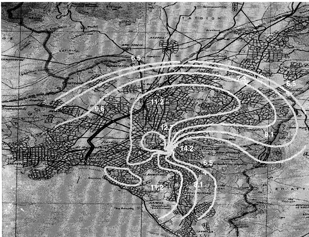
Figure 3 : Iso - Cooling load lines for the reference building in Athens for August 1996 and for 26 C set point temperature.
